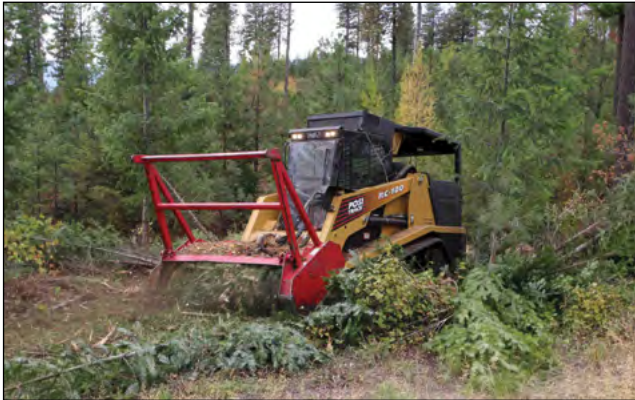
Figure 12a and 12b. Mechanical “brush mulchers” masticate ladder fuels into small chunks or chips.
