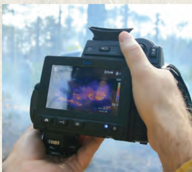
An infrared thermal camera is used to monitor surface fire behavior during a prescribed fire in north-central Florida.
