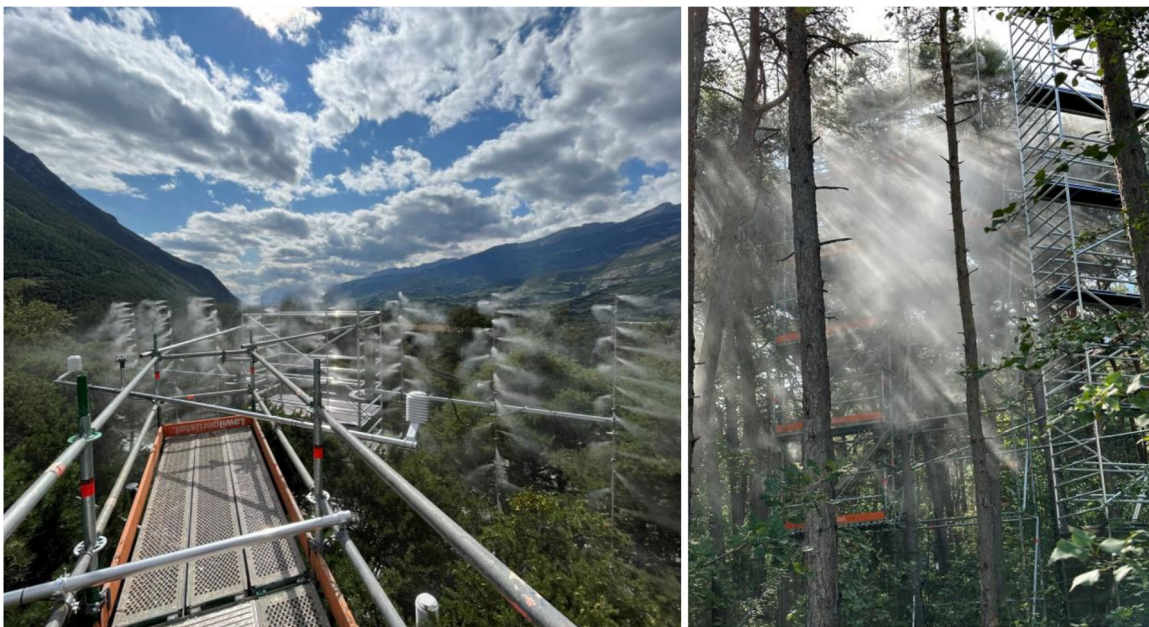
FIGURE 3 The VPDrought experiment—located near Valais, Switzerland—is the world's first atmospheric humidity and soil moisture manipulative experiment in a mature natural forest. It combines air humidity (and thus vapour pressure deficit) manipulation using a humidification system in the canopy of adult trees with soil water manipulation using a below-canopy throughfall exclusion system. Photo Credits: M. Schaub. https://www.wsl.ch/vpdrought . [Color figure can be viewed at wileyonlinelibrary.com ]
