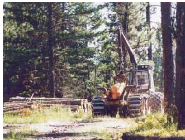
Figures 4a–b. Mechanical thinning operations. At left, a harvester performs a mechanical thinning operation in the Northern Rockies. (Andrew Youngblood, USDA Forest Service, cfc.umt.edu ) At right, a forwarder works at the Blue Mountain FFS site in northeast Oregon. (Elizabeth Dodson Coulter)
