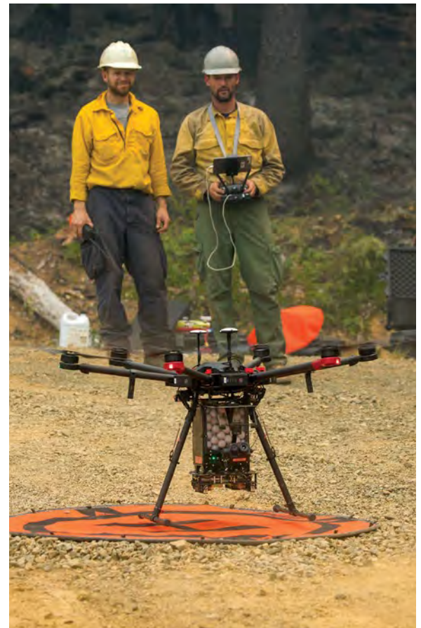
Operators launch Plastic Sphere Dispensers (PSD) from a drone to ignite a burnout operation while fighting the Klondike and Taylor Creek fires. Photo: Kari Greer/for the USDA Forest Service Pacific Northwest Region
