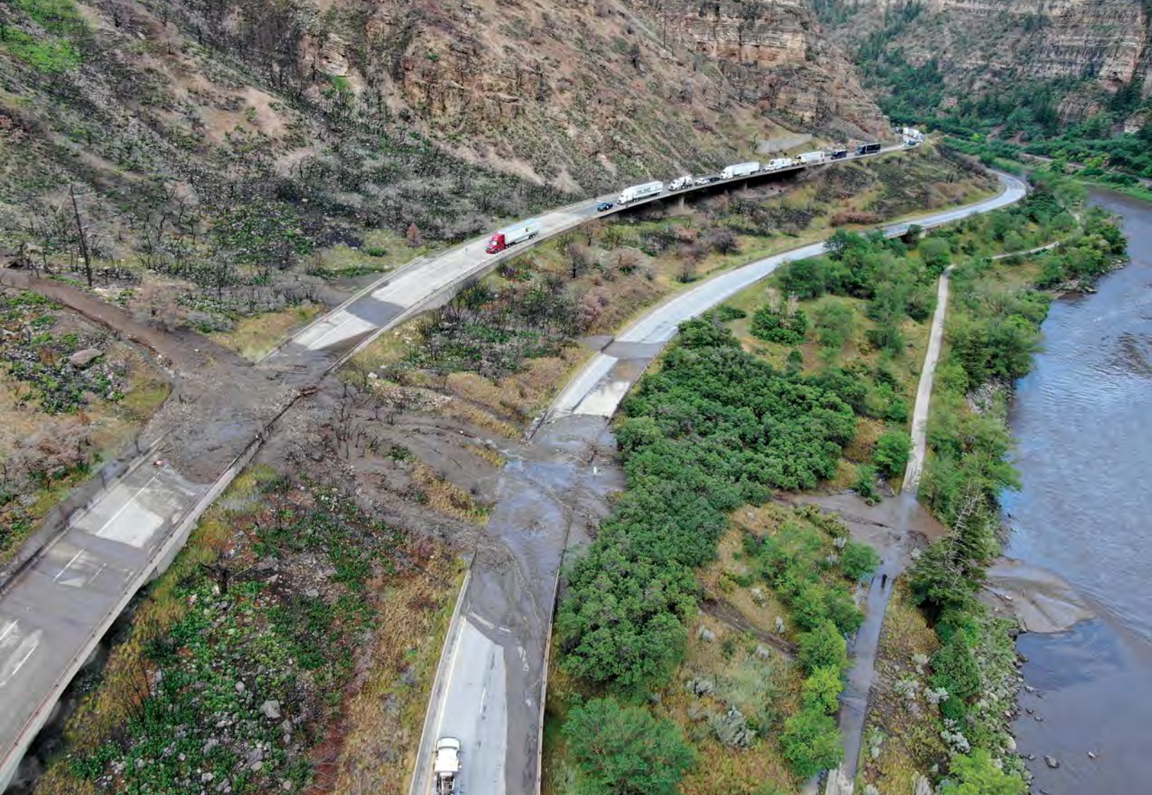
Numerous post-fire mudslides in 2021 closed sections of Interstate 70, the national transportation route that weaves through Glenwood Canyon in the mountains of Colorado. Some detours added up to four hours for travelers after the interstate was repeatedly shut down following the Grizzly Creek Fire of 2020. Photo: Glenwood Springs Fire Department
