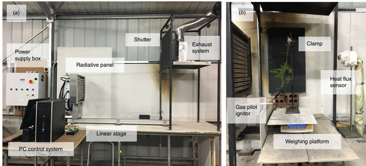
Fig. 1. (a) Full view of the VHFlux and (b) closer view of area where ignition takes place.
