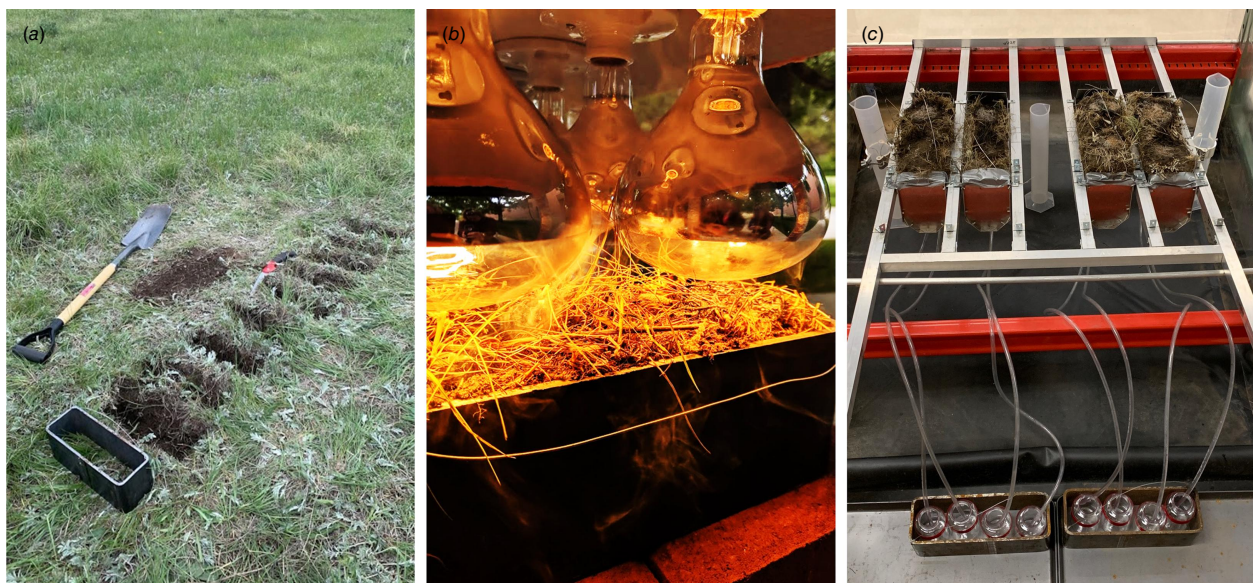
Fig. 2. The steps involved in the simulation experiment process. (a) Excavating soil samples, (b) heating in the wildfire simulator, and (c) applying precipitation in the rainfall simulator (water quality analyses not pictured). Photos courtesy of Carli Brucker.
