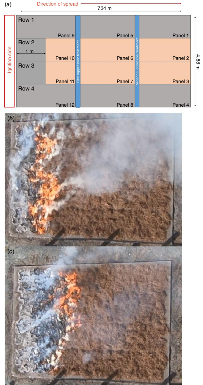
Fig. 3. (a) Layout of the burn pad that depicts each ‘row’ on the burn platform (Fig. 1b rotated 90° clockwise). Most of the experimental fires were ignited along the leftmost edge from top to bottom and spread to the right. Rows 1 and 4 were removed from fire behaviour analysis to eliminate any potential edge effect. The first 1 m strip of pixels where ignition occurred was removed from analysis to remove surges in fire behaviour during ignition. The inner two rows (row 2 and row 3) were treated as separate burns. (b) Example of a burn (B9) showing fire behaviour before suppression, and (c) immediately after indirect suppression was applied.
