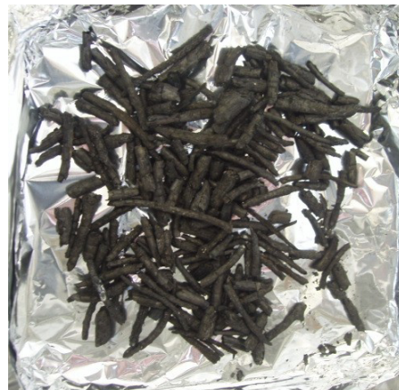
Figure 4 Digital picture of the firebrands produced from the firebrand generator. These images are taken after the firebrands were extracted from the water filled collection pans and dried.
