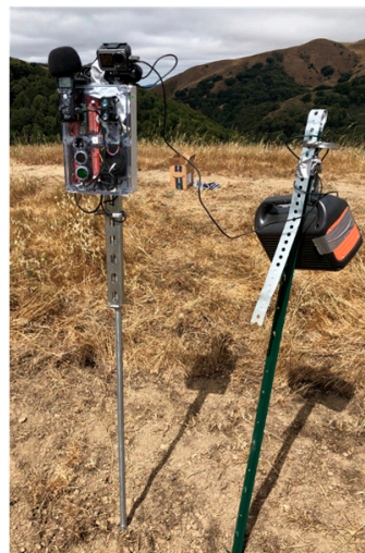
Figure 3. A picture of a deployed sensor system that included the sensing unit (left) and a backup power supply (right). Both subsystems were mounted above ground level to limit the fire exposure.
