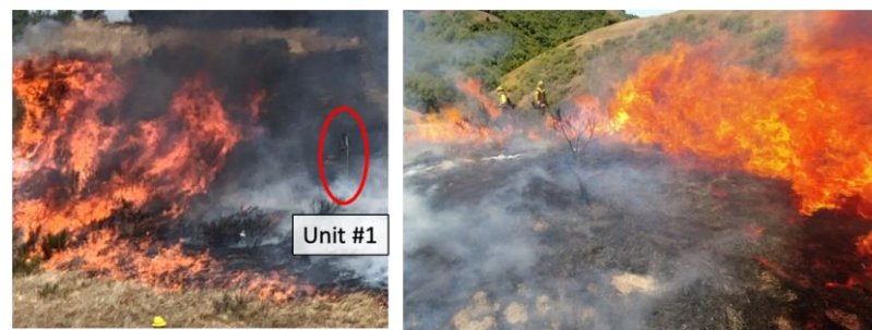
Figure 4. Unit 1's first experimental trial seen by the external observer ( left ) and by the camera mounted on the in situ sensor ( right ).
