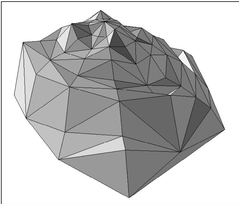
Figure 6—Example triangular irregular network lattice for a typical pile at the Naches, Washington, field site. This pile was 0.73 m high and 1.86 m wide; the “true” volume of this pile was 1.08 m<sup>3</sup>.
