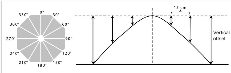
Figure 5—Overhead plan view (left) and cross-section view (right) of pile surface measurement methodology.
