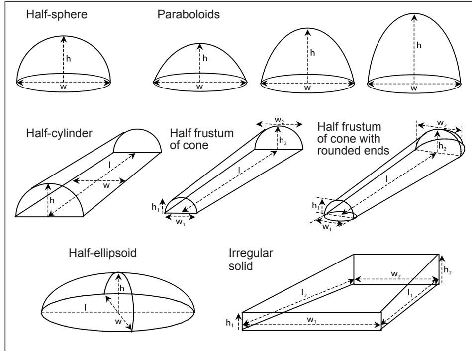
Figure 4—Geometric pile shapes and required dimensions. Redrawn from Hardy (1996).
