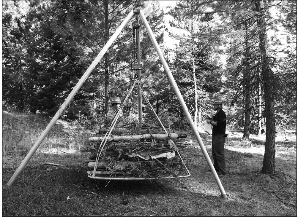
Figure 3—Pile suspended from tripod during periodic remeasurement.
