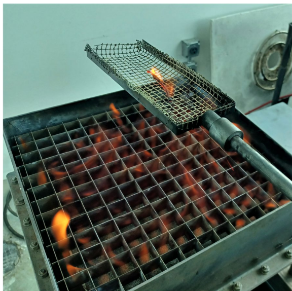
Fig. 3 A photo of the open flame burner used to conduct ignition and consumption tests. Branchwood segments were held over the flames in a wire basket while time to ignition was measured
