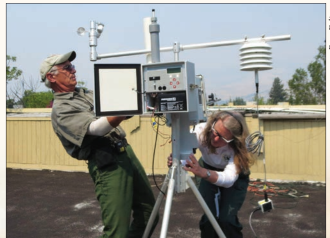
Janice Peterson and Gary Curcio, both air resource advisors, install an air quality monitor on the roof of a theater in Ashland, Oregon in 2015.
